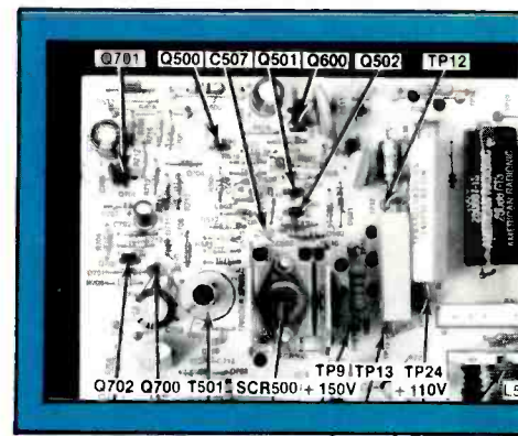
Figure 7. Regulator components and test points are identified on the power/horizontal circuit board.
